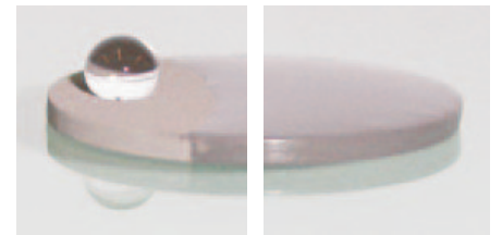
Sandblasted and thermal acid-etched model substrate with water on the unconditioned(left) and conditioned(right) surface
